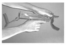
(a) Install Cocking Knob. Retract bolt until slot in bolt aligns with the rear of the slot in the upper receiver. Slide in cocking knob until it seats. Slide bolt and cocking knob forward.
