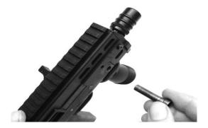
③ Pull lower receiver back about an 1/8", then pull trigger and hold. While holding trigger back, pull lower receiver downward and back to remove.
